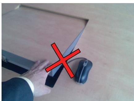
**Don't trap wires in the flip mechanism!!**
