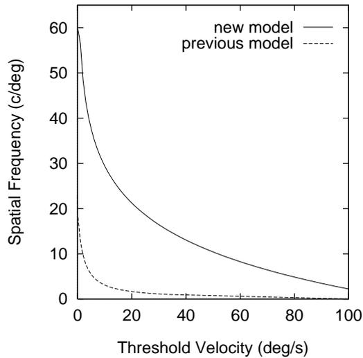
Figure 9: *Comparison between our new and previous definitions for the spatiotemporal threshold surface. The solid curve represents our new empirically derived model (Equation 20), whilst the broken curve represents our previous definition (using Equation 6).*
