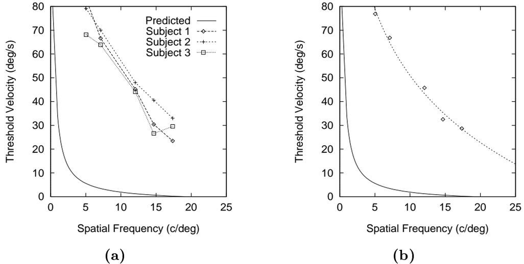
Figure 8: *Results of the velocity experiment. (a) presents the individual responses of each of the three subjects, while (b) presents the averaged response for all subjects (the data points) and the best fit curve to this average response (the dotted line: Equation 18). The continuous line in (a) and (b) represents the predicted response from our model.*
